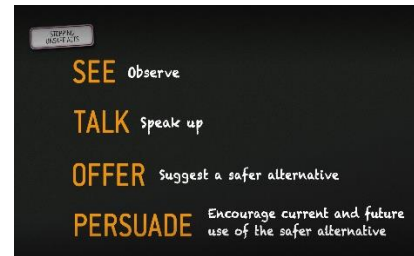
'STOP' ways to stop unsafe acts (Check out the Stopping Unsafe Acts animation and game )
